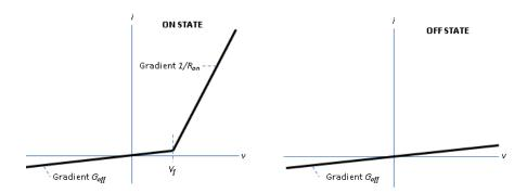
The GTO turns on if the gate-cathode voltage exceeds the specified gate trigger voltage. The device turns off if the gate-cathode voltage falls below the specified gate turn-off voltage value, or if the load current falls below the specified holding-current value.
