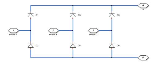
Using the Charge Dynamics tab of the block dialog box, you can choose the type of diode that the three-arm bridge circuit uses. The table shows you how to set the **Model dynamics** parameter based on your goals.
