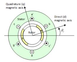
The rotor magnetic field due to the permanent magnet(s) creates a sinusoidal rate of change of flux with rotor angle.
